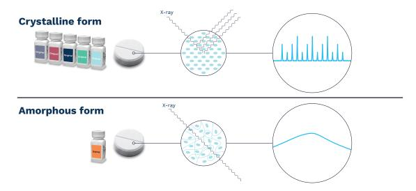
The illustration shows how different a crystalline structure is compared to an amorphous one. The crystalline structure shows a clear, regular pattern, the amorphous shape is disordered, while maintaining its stability and properties. A X-ray shows peaks in a crystalline structure, in an amorphous structure such peaks are missing.
